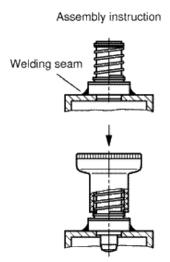
To prevent damage of the plastic knob, it will be driven onto the shaft using a plastic mallet, after the welding process.
